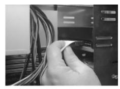
If you are replacing your CD-ROM: connect DVD-ROM to the SCSI interface connector that the CD-ROM was connected to.
